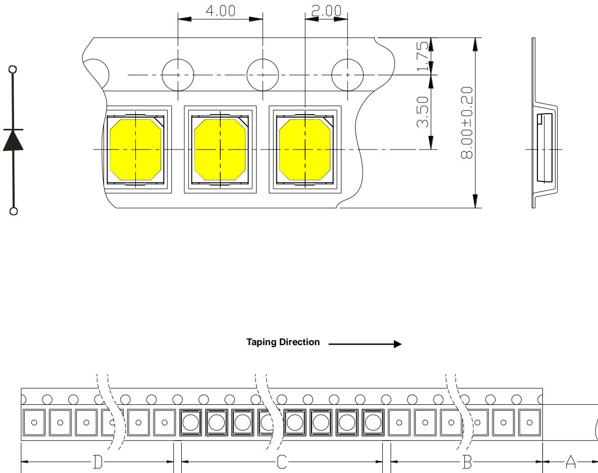
A: Top Cover Tape, 300mm; B: Leader, Empty, 200mm; C: 4000 Lamps Loaded; D: Trailer, Empty, 200mm.
